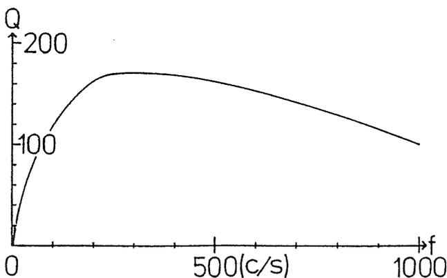
Fig. 6: Typical quality factor for the prototype reactor Fig. 5
