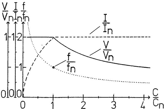
Fig. 2: Operating characteristics of circuit acc. to Fig. 1
