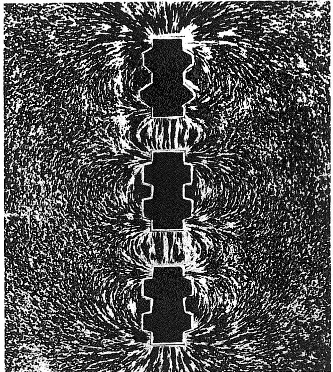
Fig. 4: Magnetic flux distribution for three reactor units
