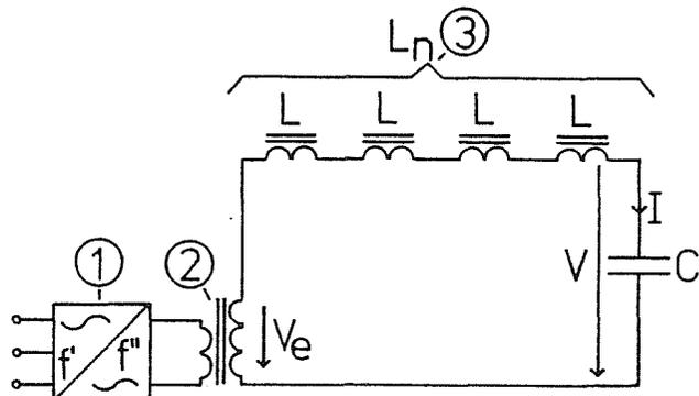
Fig. 1: Schematic diagram of SR-test circuit
