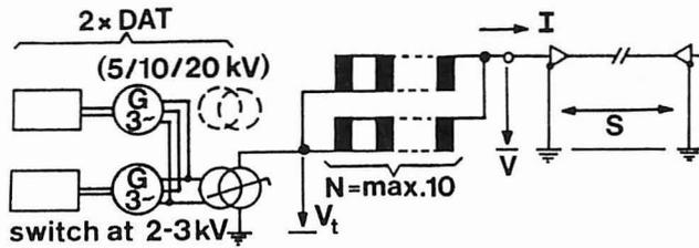
Fig. 3 . Cable-Test Connections with Single-Stage Reactors for Short Test Duration,  $T = 1 \dots 5$  min.
