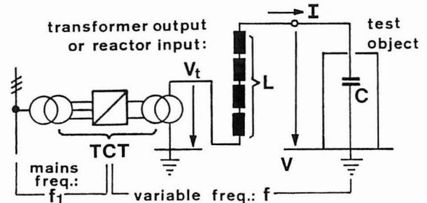
Fig.1. First Frequency-Tuned Series Resonant Test Circuit.
