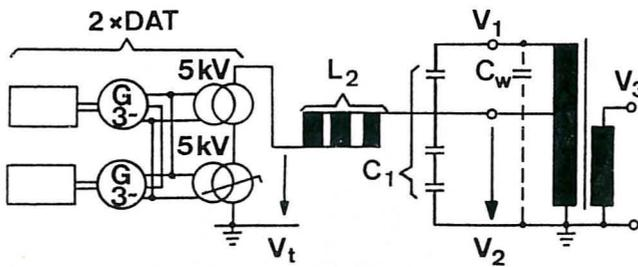
Fig. 5 . No-Load Test of an Auto-Excited Transformer, Transformer Rating  $P = 100$  MVA Single-Phase,  $550/\sqrt{3} - 230/\sqrt{3} - 13.8$  kV, Consumption about 400 kVA/80 kW at 15 kV, 60 Hz Tertiary Input.
