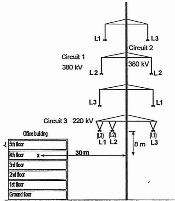
Fig. 9 Office building near transmission line
