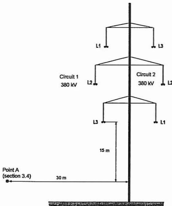
Fig. 3 Tower with optimal phase arrangement
