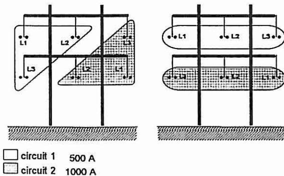
Fig. 10 Possible grouping of the phase conductors
