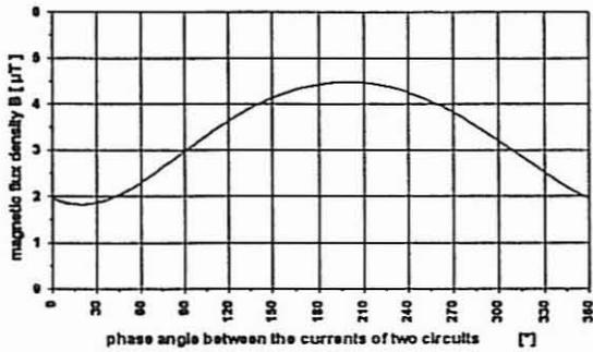
Fig.7 Magnetic field for varying phase angle difference 2 circuits, 1000 A each, configuration see fig. 3
