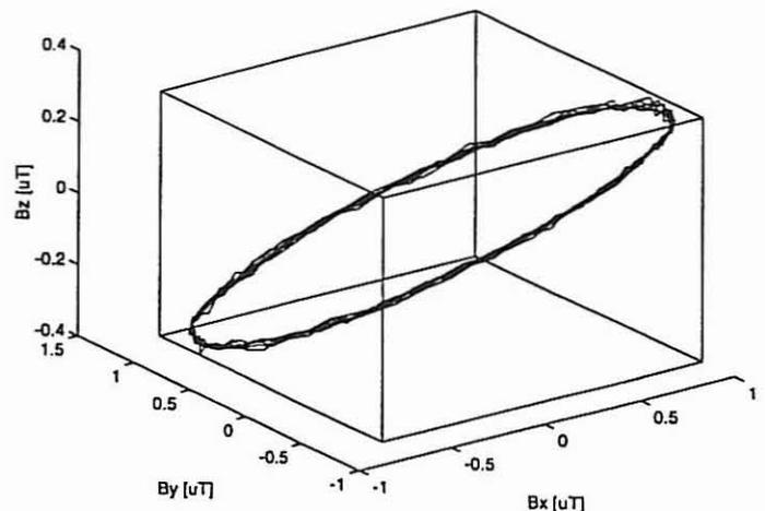
Fig. 2 Vector locus (measured),  $B_{RMS} = 0.941 \mu\text{T}$
