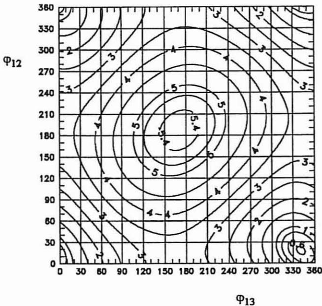
Fig. 8 Magnetic field of three circuits with varying phase angles (values in  $\mu\text{T}$ )
