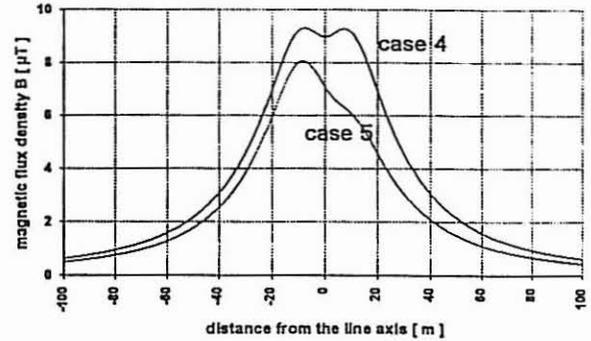
Fig. 6 Magnetic fields for reverse power flow
