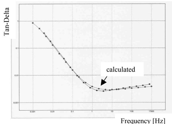
Figure 2 - Measured and calculated loss tan delta in a large autotransformer, 400 MVA, 400/220 kV (FDS-method)
