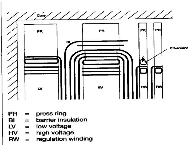
Figure 3 – PD-source in the insulating system
