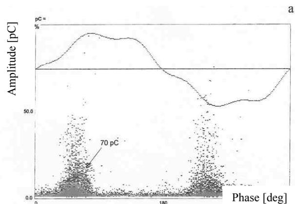
Figure 4 – PD-pattern at the 220 kV bushing of a 400 MVA autotransformer.
