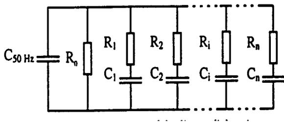
Figure 1 - Theoretical model of linear dielectrics,  $R_0$  = DC resistance,  $R_i$ ,  $C_i$  = individual elements,  $C_{50\text{Hz}} = \epsilon_r \cdot C_0$
