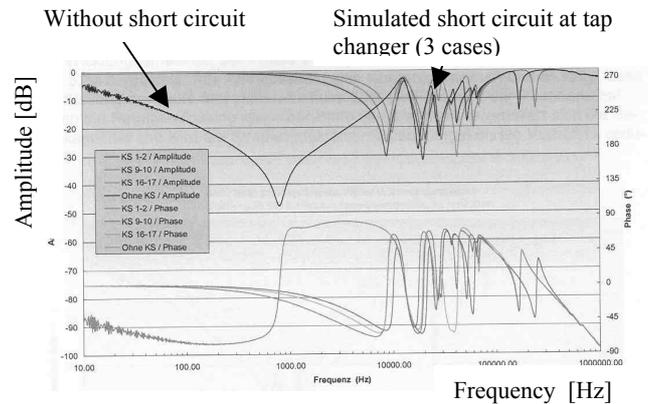
Figure 6 - Example of FRA-measurement with short circuit at the tap changer (regulating winding of a 220/49 kV unit)
