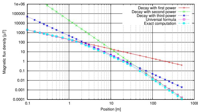
Figure 4. Decay of the magnetic flux density of a model conductor section according to Fig. 3 in the direction of point „P”. The light blue curve shows the precise calculation. The violet trace marked by squares is the result of eq. (9). The traces of the functions (10) represent lines with different slope in the semi-logarithmic plot
