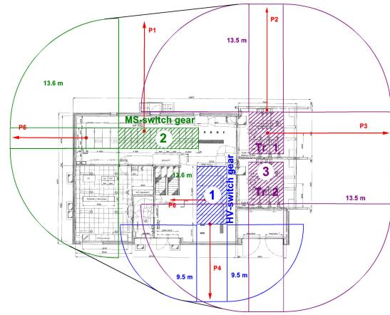
Figure 6. Result of a magnetic stray flux evaluation in a substation. The sum of maximum possible magnetic dipole moments for HV and MV switchgear and the transformers have been evaluated. The radius for the flux density to meet the emission limit of  $1 \mu\text{T}$  is plotted around the active installations
