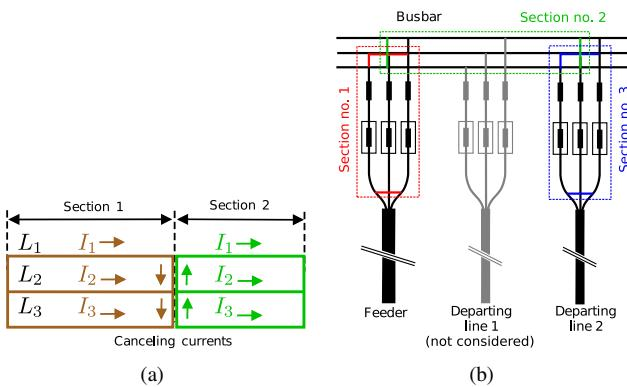
Figure 5. (a) Division of a three-phase conductor system into two sections (b) Sketch of a small medium voltage switchgear. A proposal for a definition of three-phase sections (loops) is given representing the worst-case operating condition
