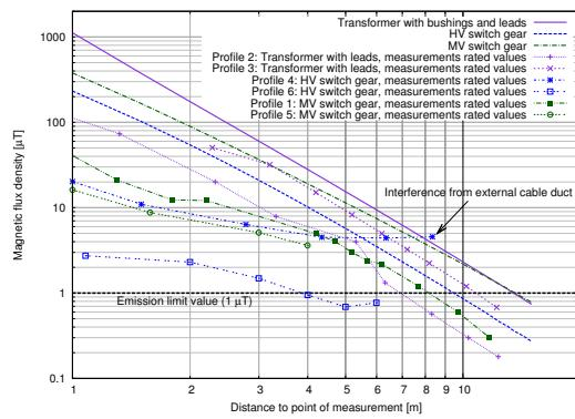
Figure 8. Theoretically evaluated and measured magnetic flux decay
