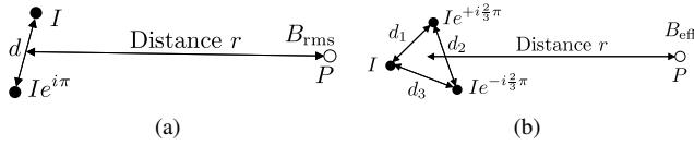
Figure 2. Definition of variables for the expression for the dipole magnetic flux density of (a) a two conductor line (eq. (5)) (b) a three-phase line (eq. (5) and (6))
