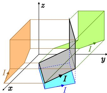
Figure 1. Projection of a non-complanate loop on three orthogonal planes
