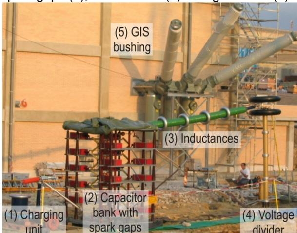
Fig. 4: Test set up for oscillating lightning impulse test at a 400-kV-GIS.
