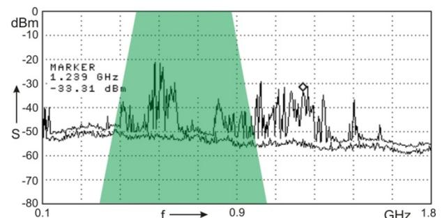
Fig. 7: Bandwidth of fixed broadband UHF method (schematic example)
