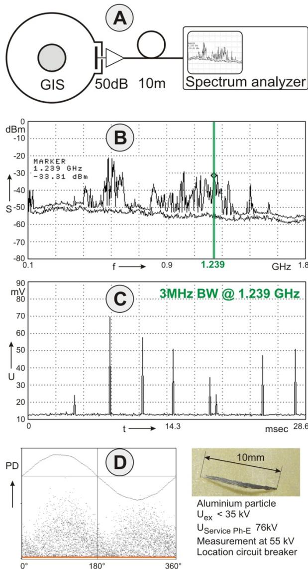
Fig. 6: Example of an tuned UHF narrowband measurement with variable centre frequency
