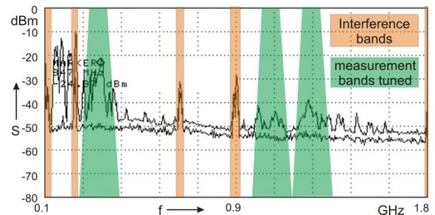
Fig. 9: Signal relationships of proposed tuned medium-band UHF method (schematic example)
