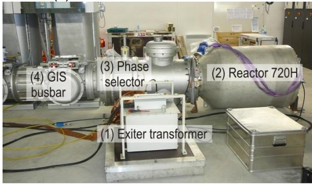
Fig. 2: Encapsulated AC resonant test set connected to a 123-kV-GIS
