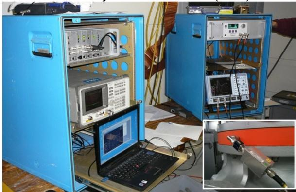
Fig. 3: PD-Measurement setup for tuned narrowband UHF-PD-measurement including time of flight measurement for PD localisation. Lower right: preamplifier attached directly to the PD sensor.
