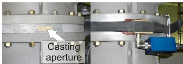
Fig. 10: Measurement with external UHF-PD-sensors: Left side casting aperture; right side PD sensor and preamplifier attached to the casting aperture
