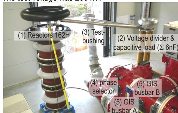
Fig. 1: AC resonant test set connected to a 123-kV-GIS
