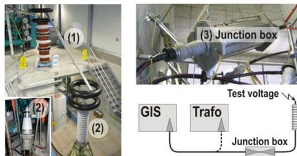
Fig. 12: Test voltage supply via pluggable test cable. Left side testing of GIS via test cable; right side testing of a cable via junction box and test cable.
