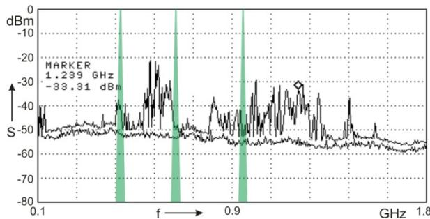
Fig. 8: Bandwidth of fixed narrowband UHF method (schematic example)
