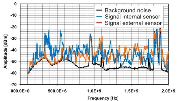
Fig. 11: Spectrum measured at an external sensor mounted at the casting aperture compared with spectrum measured at an internal sensor. PD-source: 5 pC emitted by a protrusion (needle).
