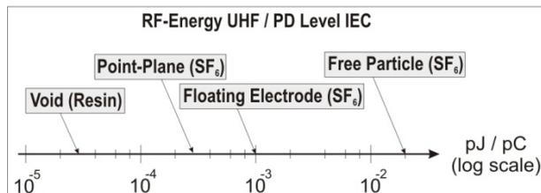
Fig. 5: Ratio of RF energy and PD level with conventional method (IEC) for different defect types [11].
